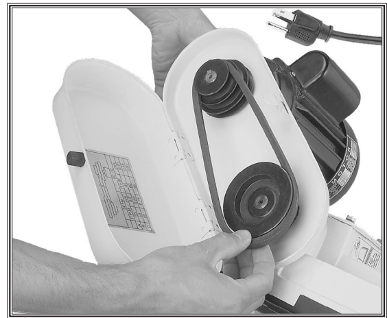
Figure 52. Installing the V-belt.
